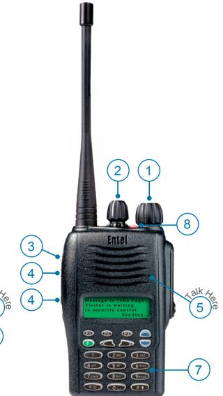
1. On/Off/Volume control. Rotate clockwise to turn on and increase volume. Rotate anti-clockwise to reduce volume & turn off.
