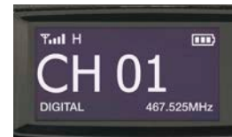
Informative display on UHF model shows both the channel number and the frequency
